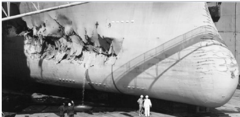
Bulk carrier Reduta Ordonea in dry dock in 1996 showing damage caused by striking an ice flow at speed in Canada's Hudson Strait in July 1996
